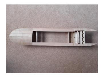
Over the next couple of months I continued adding structure to the hull, fitting the electrics, building the smoke unit and even starting planking the lower deck. Taking advantage of a sudden warm spell in April I sprayed the hull in Rover Brooklands Green followed by several coats of clear lacquer, ready for those inevitable scrapes at the pond.
