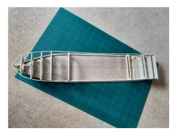
For the sides and stern of the hull I can use plywood sheet but the shape of the bow means I have to plank on frame, although, progress is good and by late January I have completed most of the hull and started planning layout of electrics.
