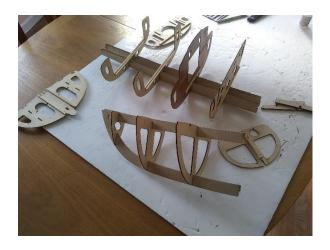
Starting with the bow section each sub-assembly was fixed in the hull and to the adjoining sub-assembly using a combination of superglue, rapid set Araldite and lengths of masking tape to hold the frames to the hull interior whilst the glue hardened.
