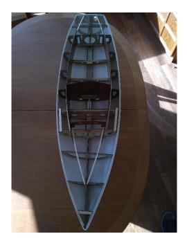
With all deck stringers installed the centreboard, after being spray painted a copper colour, was glued into place using Araldite to make a hopefully waterproof seal. The model requires an additional 1.5kg of ballast and after a long internet search loose lead shot was located on eBay at a reasonable price and 2kg have been ordered with delivery due in the next couple of days.
