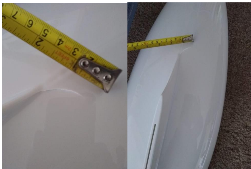
Photos showing size and location of damage to hull.
