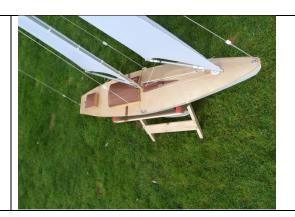
Rear deck fitted and glued in place. At this time I decided to add cabins to the rear deck and make it into a 1930 type sailing yacht. I decided not to use the normal sticky plastic racing pads as I was not going to be racing and wanted the craft to look different on the water.
