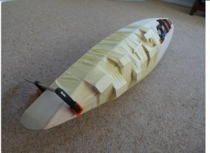
As I had a sheet of Alloy in the garage I made the dagger board from it, but still cut to the ordinal shape. I made a special frame as the one shown on the drawing was for a thicker, removable dagger board as in the 1 metre regulations. The base can now be glued on with lots of masking tape and blocks to hold the planks against the frame. At this point I admit that I made a mistake by not using narrower planks on the bottom but you always learn be your mistakes.
