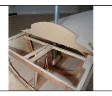
Squaring up the mast before gluing the support tube and base block in place. Using this method the mast just drops into the tube for easy transport.
