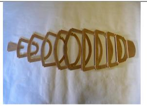
I finished the outside using files. To keep the boat light the centres were cut out using a jig saw and files. Also shown are the notches because I was going to make a frame to glue the planking against.
