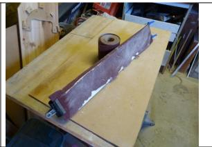
Now it's time to glue the sides on. This was made easy due the flat sides of the design that only required a single sheet of ply and lots of clamps, but you have to be careful that the ribs and frame are flat for total coverage of the glue. To achieve this flatness I use a long flat board and a length of abrasive paper with clips at either end which is nearly as long as the boat. This helps to remove any high spots over a long length easily.
