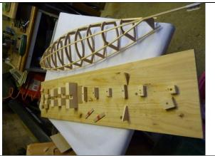
After gluing the assembly can be lifted off the jig and checked for squareness. It's better to check at this stage when adjustments can be made by cutting and regluing.
