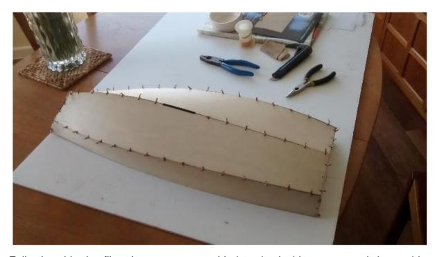
Following this the fibreglass tape was added to the inside seams and thoroughly soaked with resin. The hull was then left to dry for a couple of days before trimming off the excess copper wires as flush to the outside of the hull as possible.
