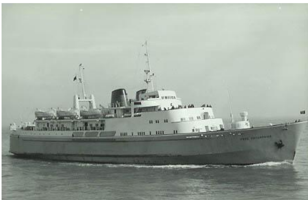
Free Enterprise I – 1966 Roll On Ferry belonging to Townsend Bros Ferries and operated on the Dover to Calais channel crossing. 96 metres in length. 120 cars on 2 decks and 6 freight vehicles
