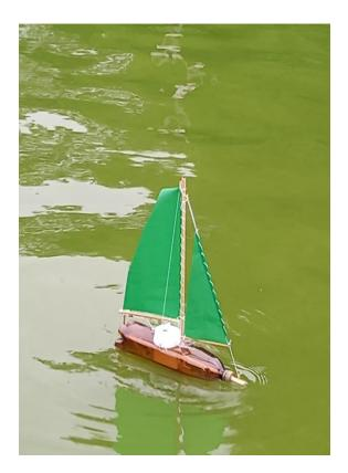
Would I change the design to make construction easier? Yes, you only find out by making mistakes and I am still not sure if you need the structural dowel going through the bottle. I would also fit the mast through the bottle and glue the dagger board onto it to save cutting the slot.
